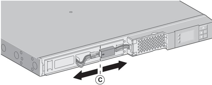
**C** - Disconnect the battery block by separating the two connectors (never pull on the wires).
