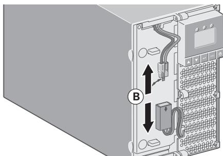
**B** - Disconnect the battery block by separating the two connectors (never pull on the wires).
