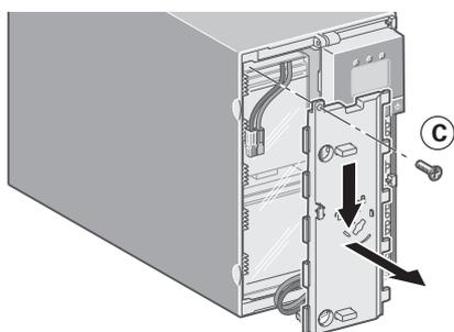
**C** - Remove the plastic protection cover in front of the battery (one screw).
