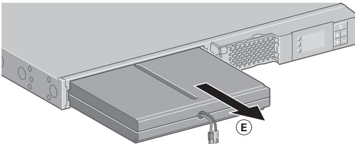
**E** - Pull the plastic tab to remove the battery block and replace it.
