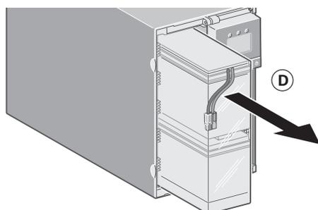
**D** - Pull the plastic tab to remove the battery block and replace it.
