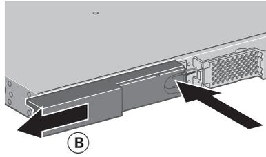
**B** - Remove the left-hand side of the front panel by pushing the button and then by sliding the part.
