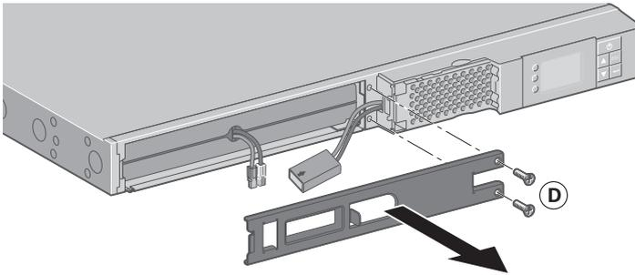
**D** - Remove the metal protection cover in front of the battery (two screws).
