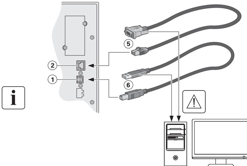
1. Connect the RS232 (5) or USB (6) communication cable to the serial or USB port on the computer equipment.
