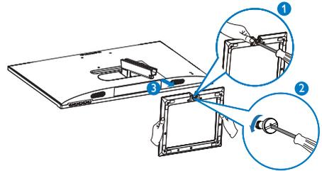
3. Remove the hinge cover from monitor body by using your fingers.
