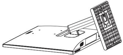
2. (1) Use a screwdriver to loosen the screw located at the bottom of the base.
