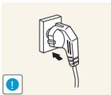
Insert the power plug all the way in so it is not loose.
