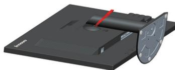
Step 3: Remove the base and stand from the monitor, refer to "Detaching the monitor base and stand" on page 2-12.
