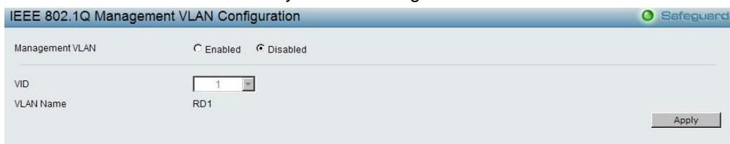
Figure 66 – Configuration > 802.1Q Management VLAN
